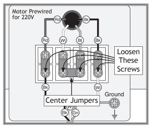
**Figure 4.** Locations of screws to be loosened.
